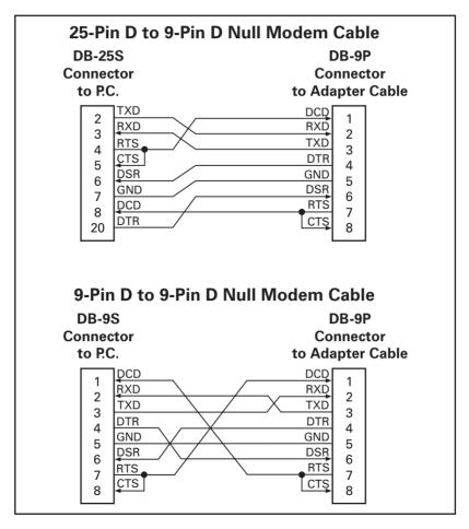
**Null Modem Cable Pinouts**
